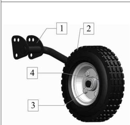
*Fig. 3: Steering Wheel Assembly*
